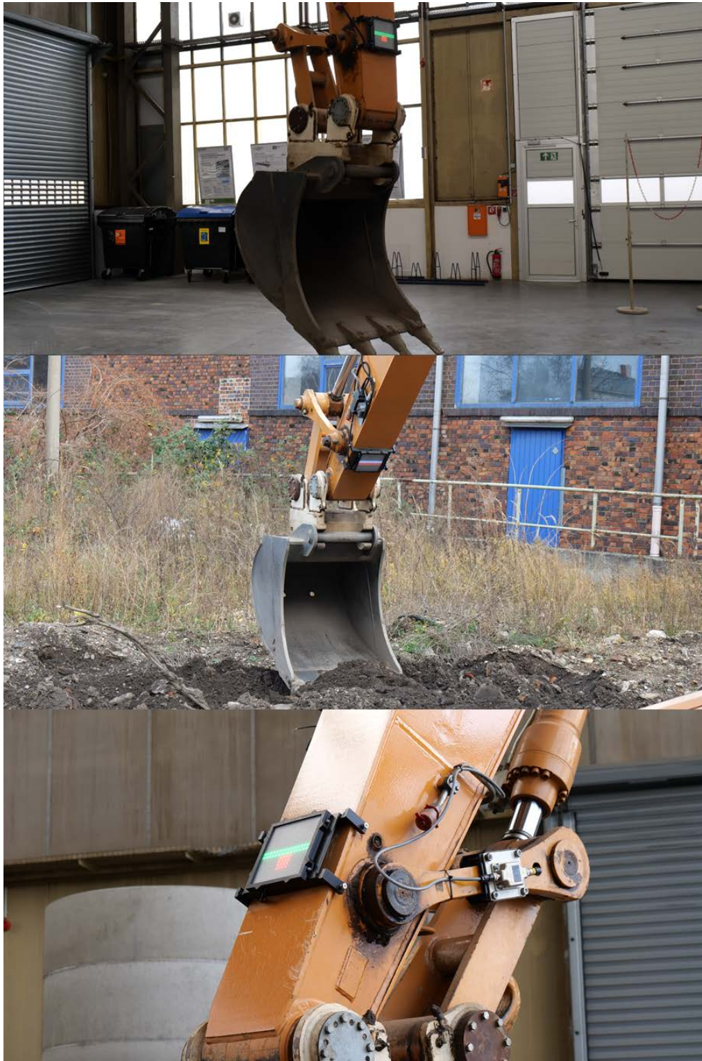
Figure 36: The LED-matrix display indicates the derivation to the target height
