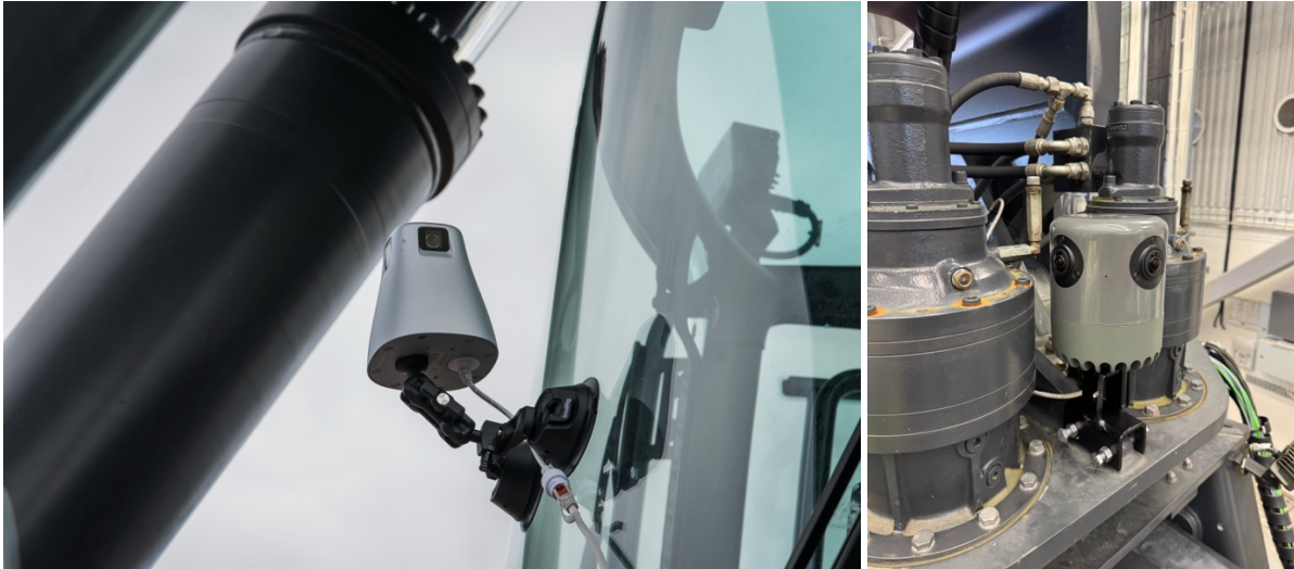
Figure 23: Nokia360 camera is mounted on top of the spreader, while Cupola360 was placed on the cabin's windshield.
