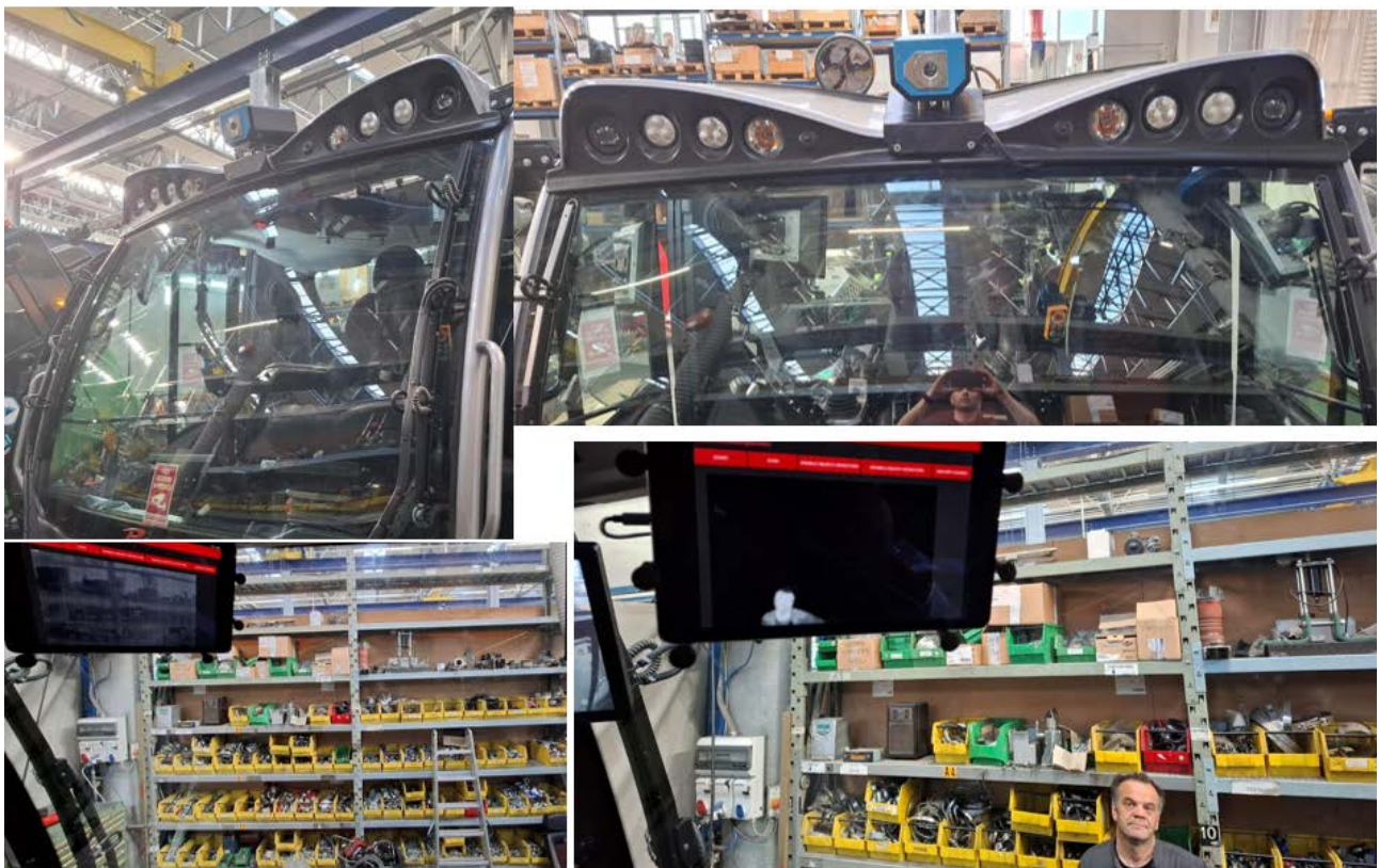
Figure 1: Installed thermal camera on a Leitwolf
