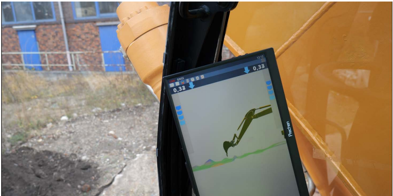
Figure 38: Sideview of the actual surface in the main display.
