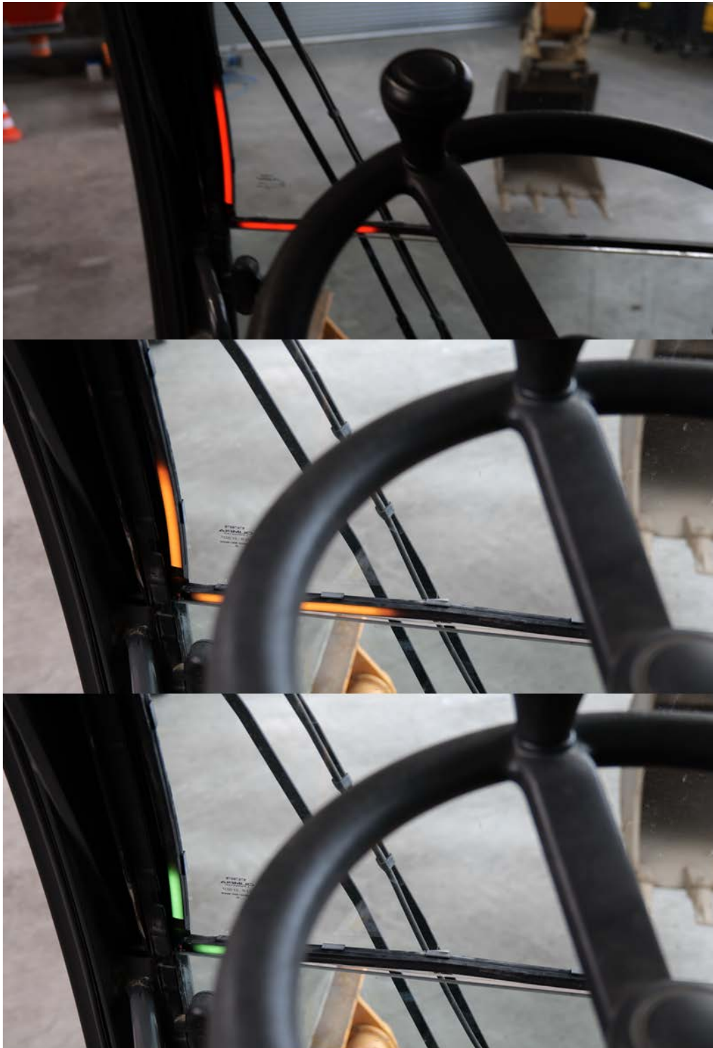
Figure 35: The LED-indicator around the front facing window visualizes the direction and distance to persons in the danger zone
