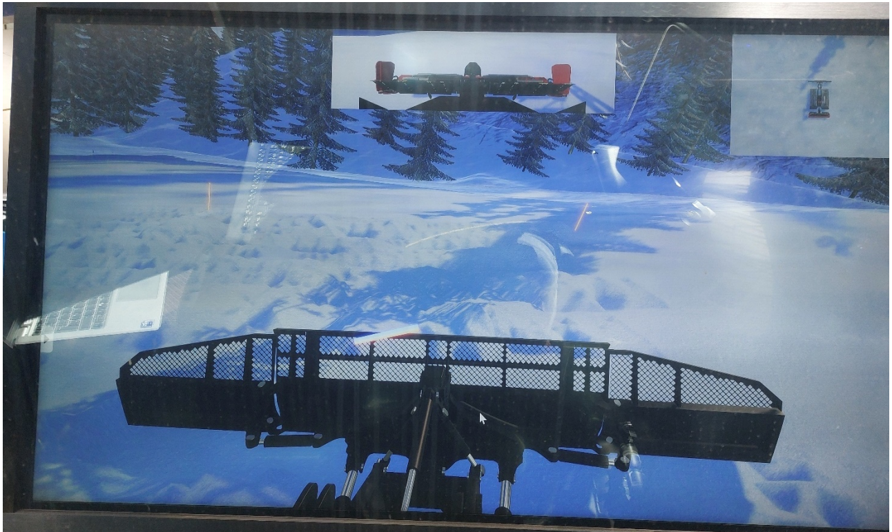
Figure 15: Indicator overlapping between blade position and target position
