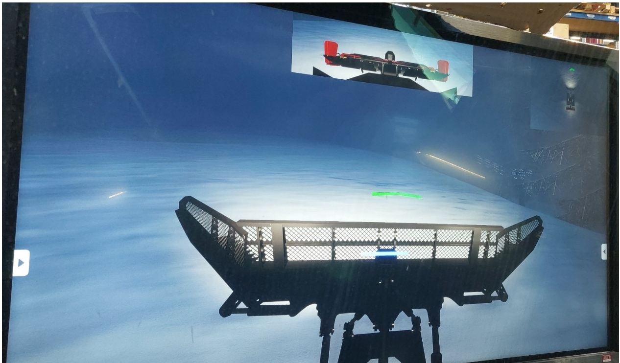
Figure 13: Simulation with rear view, 360° top view, blade indicator bar and path projections
