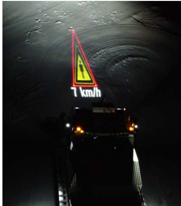
Figure 6: Person proximity projection on snow surface
