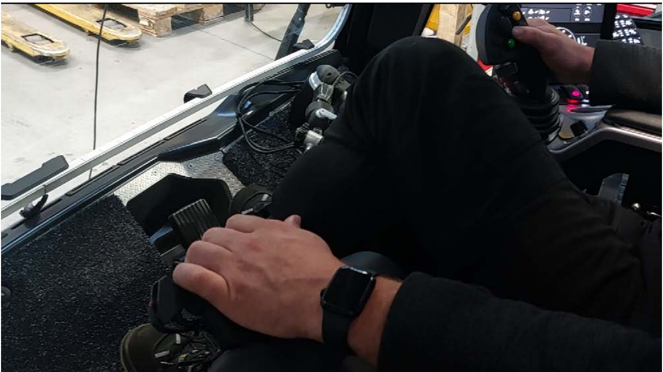
Figure 18: Cabin setup with haptic track controls
