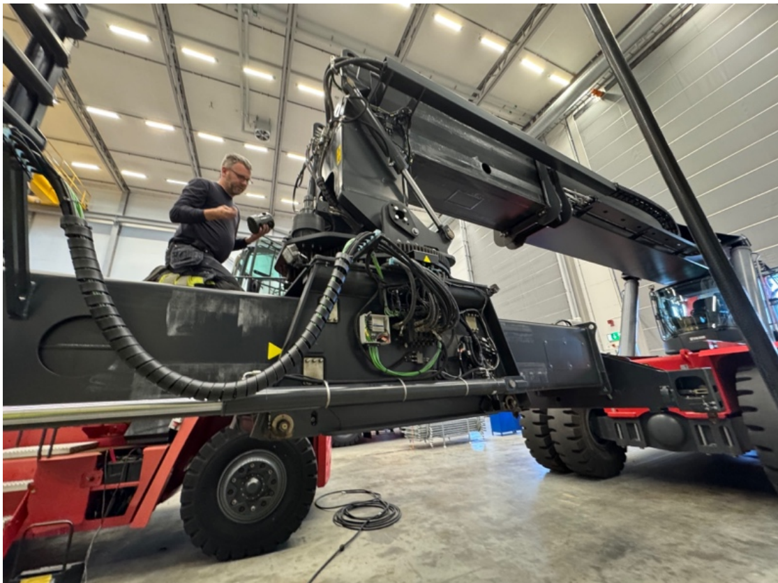
Figure 24: Personnel from Kalmar mounting the Nokia 360 camera on top of the reach stacker's spreader.
