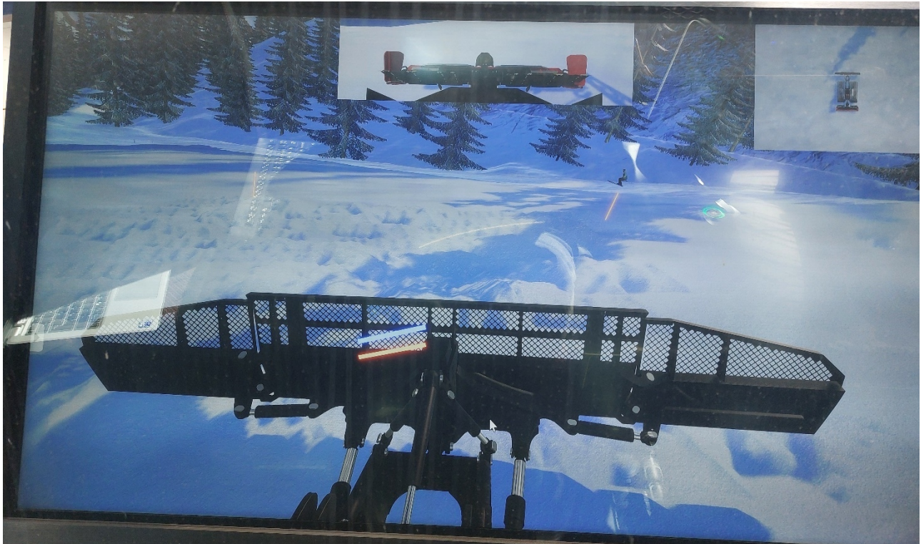
Figure 14: Target area with snow to be removed and indicator of blade position vs target position
