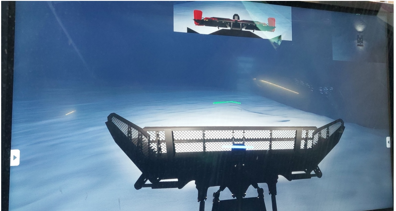
Figure 19: No view scenario with projected arrow guidance
